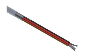
Quabbin control cable, shielded, 3 conductors, 18 AWG, 16-stranded, tinned copper, PVC conductor insulation material, PVC jacket, gray, cut to length.
