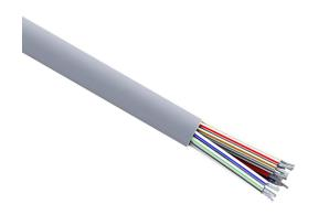
Quabbin control cable, unshielded, 25 conductors, 18 AWG, 16-stranded, tinned copper, PVC conductor insulation material, PVC jacket, gray, cut to length.
