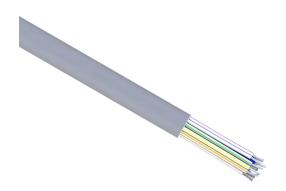
Quabbin control cable, unshielded, 19 conductors, 18 AWG, 16-stranded, tinned copper, PVC conductor insulation material, PVC jacket, gray, cut to length.
