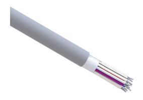
Quabbin control cable, shielded, 19 conductors, 18 AWG, 16-stranded, tinned copper, PVC conductor insulation material, PVC jacket, gray, cut to length.
