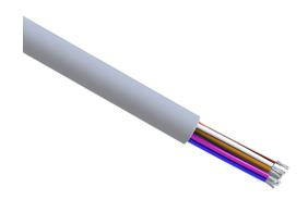
Quabbin control cable, unshielded, 15 conductors, 18 AWG, 16-stranded, tinned copper, PVC conductor insulation material, PVC jacket, gray, cut to length.
