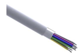
Quabbin flexible control cable, shielded, 12 conductors, 18 AWG, 16-stranded, tinned copper, PVC conductor insulation material, PVC jacket, gray, cut to length.
