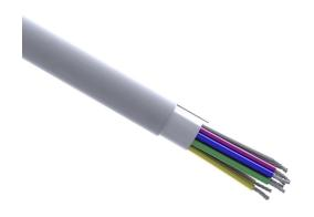
Quabbin flexible control cable, shielded, 12 conductors, 18 AWG, 16-stranded, tinned copper, PVC conductor insulation material, PVC jacket, gray, cut to length.
