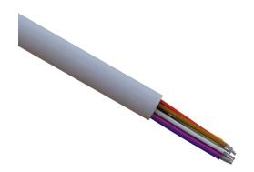
Quabbin control cable, unshielded, 9 conductors, 16 AWG, 19-stranded, tinned copper, PVC conductor insulation material, PVC jacket, gray, cut to length.
