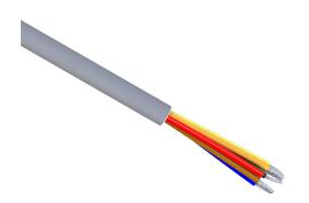
Quabbin control cable, unshielded, 7 conductors, 16 AWG, 19-stranded, tinned copper, PVC conductor insulation material, PVC jacket, gray, cut to length.
