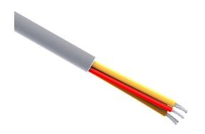
Quabbin control cable, unshielded, 5 conductors, 16 AWG, 19-stranded, tinned copper, PVC conductor insulation material, PVC jacket, gray, cut to length.
