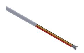
Quabbin control cable, unshielded, 4 conductors, 16 AWG, 19-stranded, tinned copper, PVC conductor insulation material, PVC jacket, gray, cut to length.
