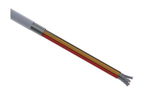
Quabbin control cable, shielded, 4 conductors, 16 AWG, 19-stranded, tinned copper, PVC conductor insulation material, PVC jacket, gray, cut to length.
