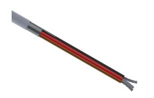
Quabbin control cable, shielded, 3 conductors, 16 AWG, 19-stranded, tinned copper, PVC conductor insulation material, PVC jacket, gray, cut to length.
