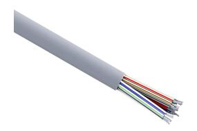
Quabbin control cable, unshielded, 25 conductors, 16 AWG, 19-stranded, tinned copper, PVC conductor insulation material, PVC jacket, gray, cut to length.
