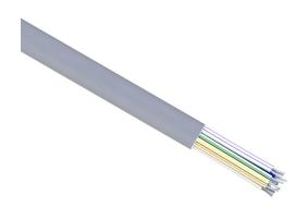
Quabbin control cable, unshielded, 19 conductors, 16 AWG, 19-stranded, tinned copper, PVC conductor insulation material, PVC jacket, gray, cut to length.
