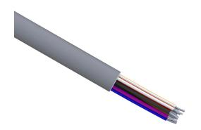
Quabbin control cable, unshielded, 15 conductors, 16 AWG, 19-stranded, tinned copper, PVC conductor insulation material, PVC jacket, gray, cut to length.
