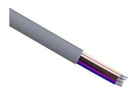
Quabbin control cable, unshielded, 15 conductors, 16 AWG, 19-stranded, tinned copper, PVC conductor insulation material, PVC jacket, gray, cut to length.
