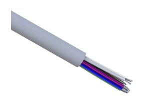
Quabbin flexible control cable, unshielded, 12 conductors, 16 AWG, 19-stranded, tinned copper, PVC conductor insulation material, PVC jacket, gray, cut to length.
