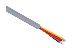
Quabbin control cable, unshielded, 7 conductors, 14 AWG, 41-stranded, tinned copper, PVC conductor insulation material, PVC jacket, gray, cut to length.
