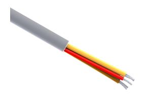
Quabbin control cable, unshielded, 5 conductors, 14 AWG, 41-stranded, tinned copper, PVC conductor insulation material, PVC jacket, gray, cut to length.
