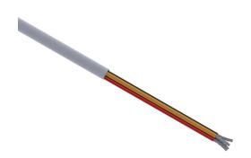
Quabbin control cable, unshielded, 4 conductors, 14 AWG, 41-stranded, tinned copper, PVC conductor insulation material, PVC jacket, gray, cut to length.
