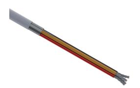
Quabbin control cable, shielded, 4 conductors, 14 AWG, 41-stranded, tinned copper, PVC conductor insulation material, PVC jacket, gray, cut to length.
