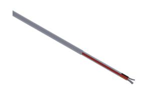
Quabbin control cable, unshielded, 3 conductors, 14 AWG, 41-stranded, tinned copper, PVC conductor insulation material, PVC jacket, gray, cut to length.
