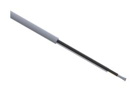
Quabbin control cable, unshielded, 2 conductors, 14 AWG, 41-stranded, tinned copper, PVC conductor insulation material, PVC jacket, gray, cut to length.
