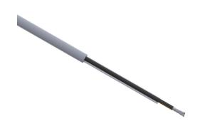
Quabbin control cable, unshielded, 2 conductors, 14 AWG, 41-stranded, tinned copper, PVC conductor insulation material, PVC jacket, gray, cut to length.
