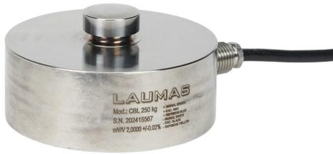
Laumas low profile compression load cell, 550 lb/250 kg, +/- 0.03% of full scale accuracy, voltage signal range(s) of 2 mV/V, 3-15 VDC, stainless steel, IP68, 16.4ft/5m integral 6-wire shielded cable.
