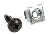
Hammond rack mounting screw, #12-24 UNF, #2 Robertson/ #2 Phillips quadrex truss head, carbon steel, black oxide finish. Package of 50. Black nylon washer and zinc-plated square-hole cage nut included.
