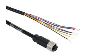
Datalogic cable, connection, M12 axial female to pigtail, 17-pole, PVC, 16.4ft/5m cable length.
