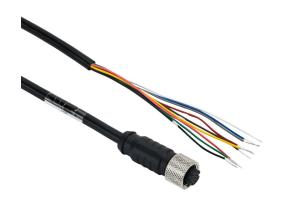
Datalogic cable, connection, M12 axial female to pigtail, 17-pole, PVC, 9.8ft/3m cable length.
