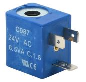
CFA solenoid coil, replacement, 24 VAC, 6.5 VA, 11mm DIN style wiring plug. For use with SC3 and SC9 series valves.
