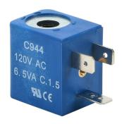
CFA solenoid coil, replacement, 120 VAC, 6.5 VA, 11mm DIN style wiring plug. For use with SC3 and SC9 series valves.
