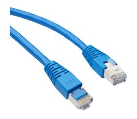
AutomationDirect Cat6a Ethernet straight-through patch cable, STP (overall foil shield), RJ45 male to RJ45 male, 10ft cable length, blue. For use with 10/100/1000/10000 Mbps networks.
