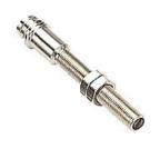
Photoelectric sensor, tubular, threaded, stainless steel housing, through-beam receiver, 250mm sensing distance, 10-30 VDC operating voltage, dark-on, PNP, 3-wire, 3-pin M8 quick-disconnect.
