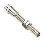
Photoelectric sensor, tubular, threaded, stainless steel housing, through-beam receiver, 250mm sensing distance, 10-30 VDC operating voltage, dark-on, NPN, 3-wire, 3-pin M8 quick-disconnect.
