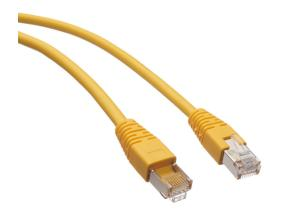
AutomationDirect Cat5e Ethernet straight-through patch cable, STP (overall foil shield), RJ45 male to RJ45 male, 50ft cable length, yellow. For use with 10/100/1000 Mbps networks.
