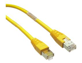
AutomationDirect Cat5e Ethernet crossover patch cable, STP (overall foil shield), RJ45 male to RJ45 male, 7ft cable length, yellow. For use with 10/100 Mbps networks.
