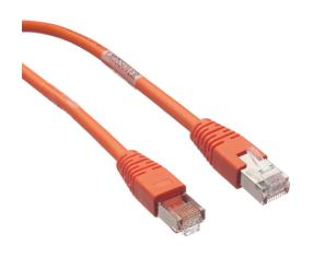
AutomationDirect Cat5e Ethernet crossover patch cable, STP (overall foil shield), RJ45 male to RJ45 male, 7ft cable length, orange. For use with 10/100 Mbps networks.
