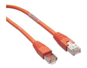
AutomationDirect Cat5e Ethernet crossover patch cable, STP (overall foil shield), RJ45 male to RJ45 male, 3ft cable length, orange. For use with 10/100/1000 Mbps networks.
