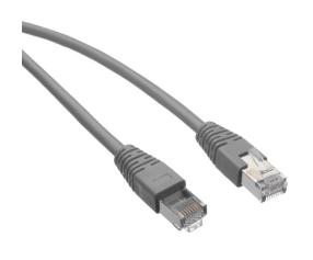
AutomationDirect Cat5e Ethernet straight-through patch cable, STP (overall foil shield), RJ45 male to RJ45 male, 50ft cable length, gray. For use with 10/100/1000 Mbps networks.
