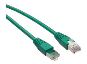
AutomationDirect Cat5e Ethernet straight-through patch cable, STP (overall foil shield), RJ45 male to RJ45 male, 3ft cable length, green. For use with 10/100/1000 Mbps networks.
