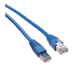
AutomationDirect Cat5e Ethernet straight-through patch cable, STP (overall foil shield), RJ45 male to RJ45 male, 7ft cable length, blue. For use with 10/100/1000 Mbps networks.
