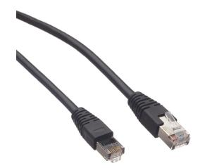
AutomationDirect Cat5e Ethernet straight-through patch cable, STP (overall foil shield), RJ45 male to RJ45 male, 50ft cable length, black. For use with 10/100/1000 Mbps networks.
