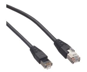
AutomationDirect Cat5e Ethernet straight-through patch cable, STP (overall foil shield), RJ45 male to RJ45 male, 14ft cable length, black. For use with 10/100/1000 Mbps networks.
