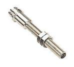
Photoelectric sensor, tubular, threaded, diffuse, infrared light emission, 50mm sensing distance, light-on, PNP, 250 Hz switching frequency, stainless steel housing, 3-pin M8 quick-disconnect.
