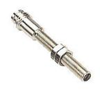
Photoelectric sensor, tubular, threaded, diffuse, infrared light emission, 50mm sensing distance, light-on, NPN, 3-wire, 3-pin M8 quick-disconnect.
