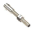
Photoelectric sensor, tubular, threaded, diffuse, infrared light emission, 50mm sensing distance, light-on, NPN, 250 Hz switching frequency, stainless steel housing, 3-pin M8 quick-disconnect.
