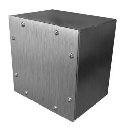
Hammond enclosure, NEMA 3/4X/12, 8 x 8 x 6in (HxWxD), wall mount, 304 stainless steel, #4 brush finish, screw cover.
