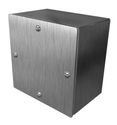
Hammond enclosure, NEMA 3/4X/12, 6 x 6 x 4in (HxWxD), wall mount, 304 stainless steel, #4 brush finish, screw cover.
