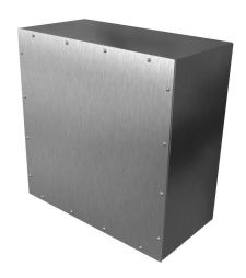
Hammond enclosure, NEMA 3/4X/12, 24 x 24 x 12in (HxWxD), wall mount, 304 stainless steel, #4 brush finish, screw cover.
