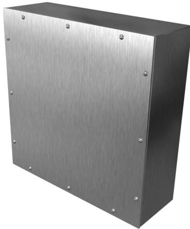
Hammond enclosure, NEMA 3/4X/12, 18 x 18 x 6in (HxWxD), wall mount, 304 stainless steel, #4 brush finish, screw cover.
