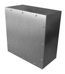
Hammond enclosure, NEMA 3/4X/12, 16 x 16 x 8in (HxWxD), wall mount, 304 stainless steel, #4 brush finish, screw cover.
