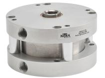
NITRA pneumatic cylinder, compact, 3in bore, 3/4in rod diameter, 1in stroke, double acting, counter-bored holes mount.
