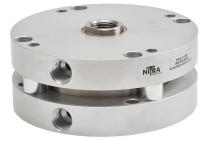
NITRA pneumatic cylinder, compact, 3in bore, 3/4in rod diameter, 1/2in stroke, double acting, counter-bored holes mount.
