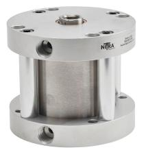
NITRA pneumatic cylinder, compact, 2-1/2in bore, 3/4in rod diameter, 2in stroke, double acting, counter-bored holes mount.
